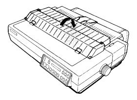
**12.** Press the **LOAD/EJECT** button to feed the paper to **the** loading position.
